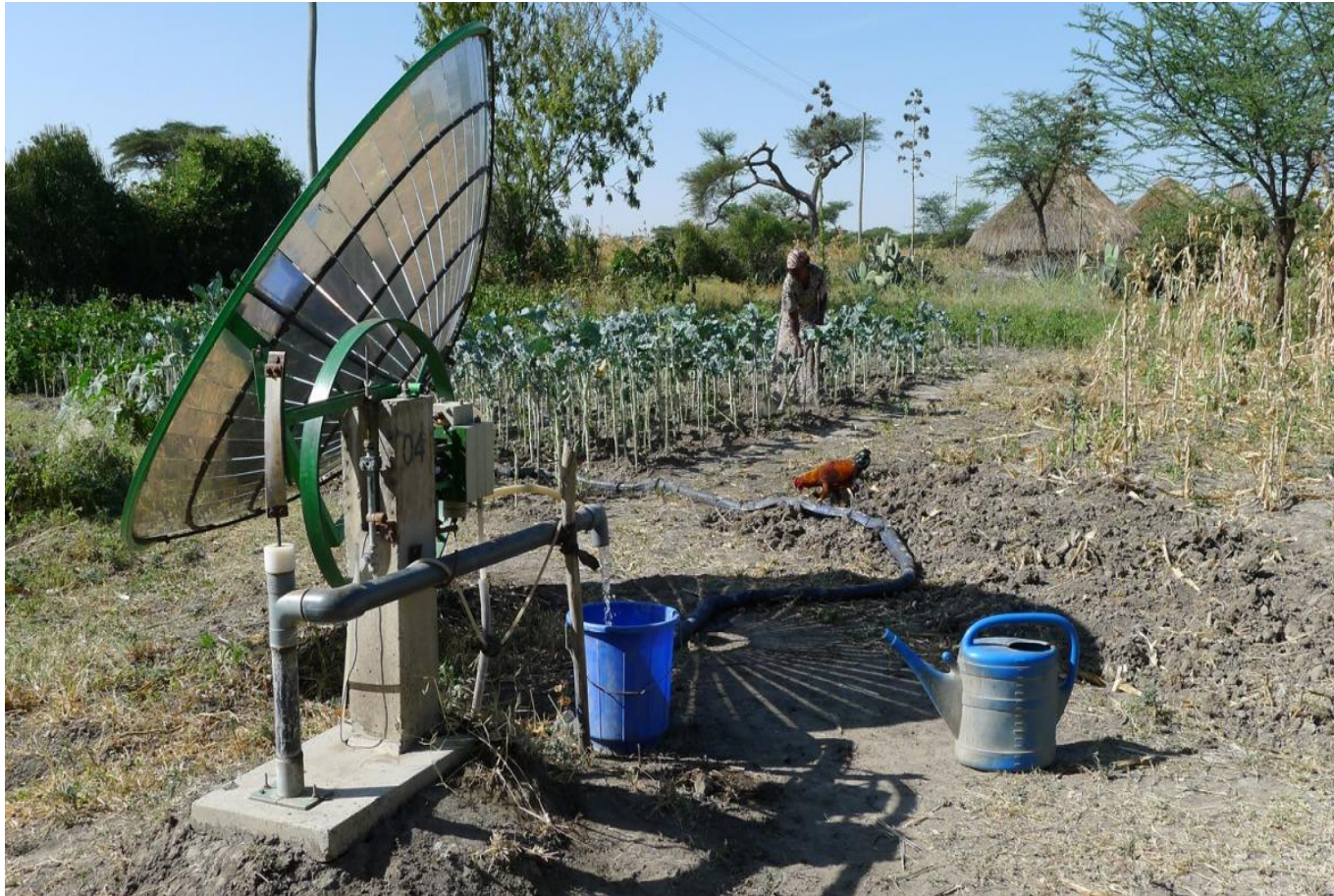
Solar steam generator and steam engine that operates with a high efficiency for pumping water
