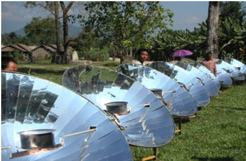
Parabolic type solar cooker
